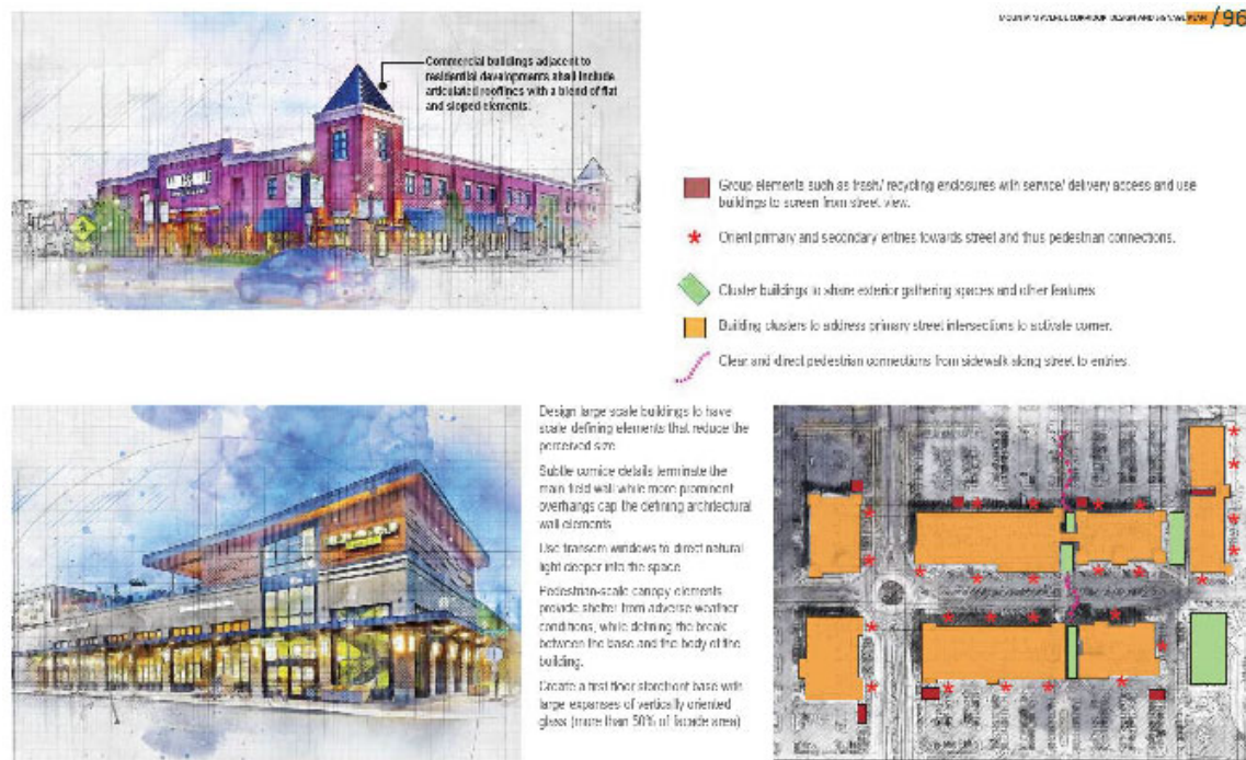
Figure 3.23: Massing for Buildings 75' in width or larger
