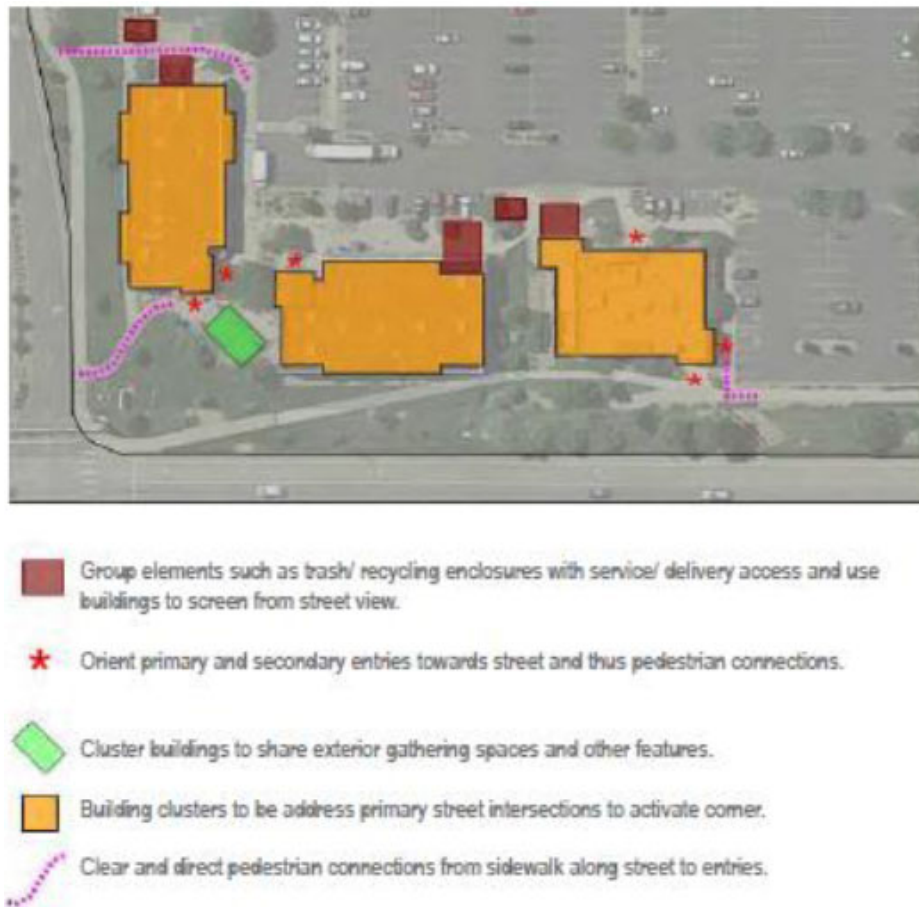
Figure 3.9: Building Placement Example
