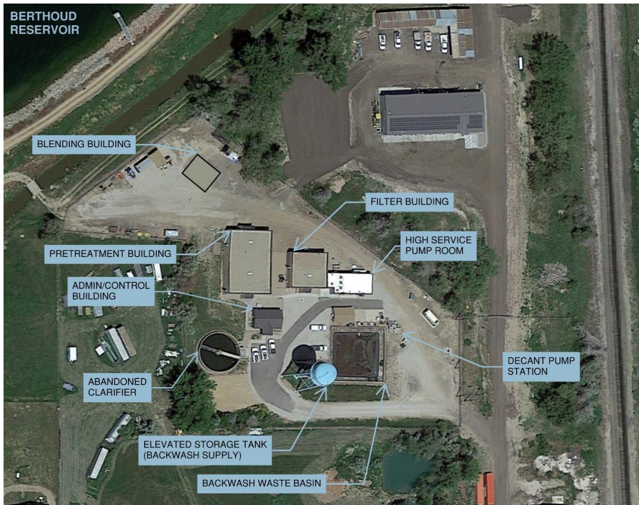
Figure 4-2: Berthoud WTP Site Arrangement
