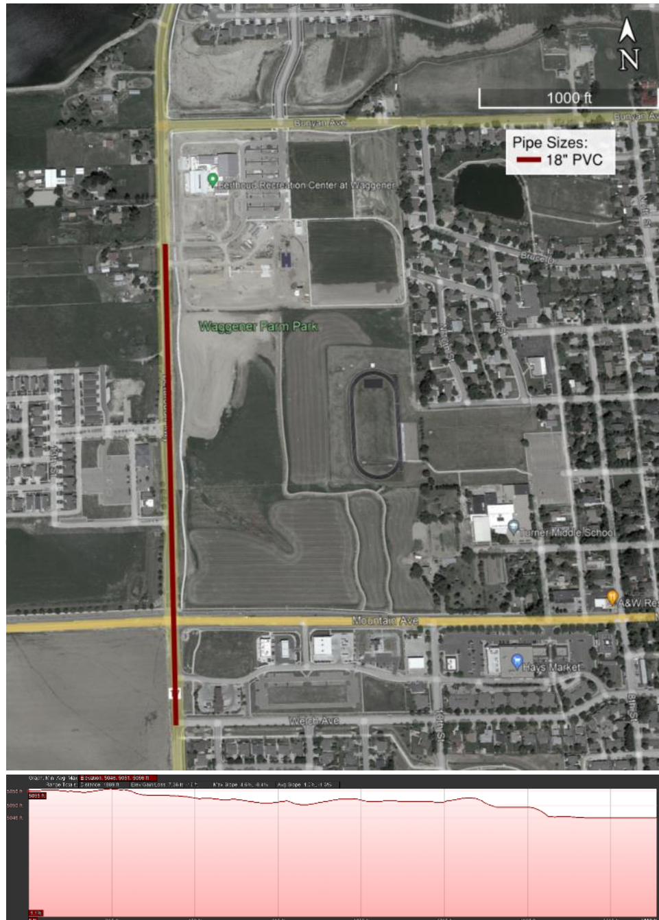
Figure 5-24: WWC-4: Berthoud Parkway Trunk Sewer
